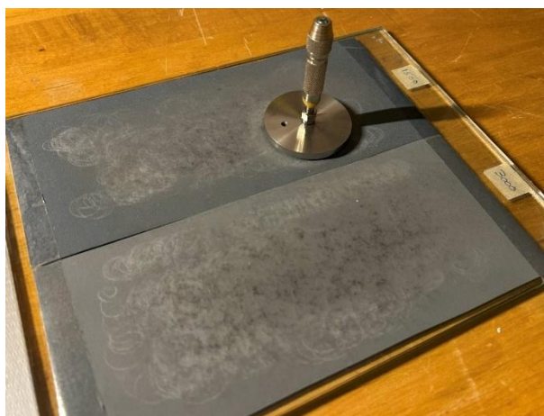
Figure 1. Aluminum puck fiber holder and grit paper.
