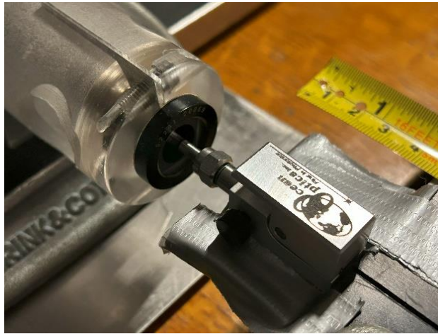
Figure 5. Close up of the fiber chuck against the photodiode window.
