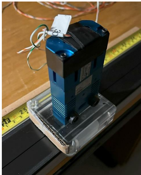
Figure 6. UV LED housing and acrylic runner.
