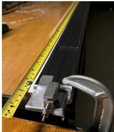
Figure 4. Fiber testing tray (puckboard) showing the 1mm-diameter groove along its length.
